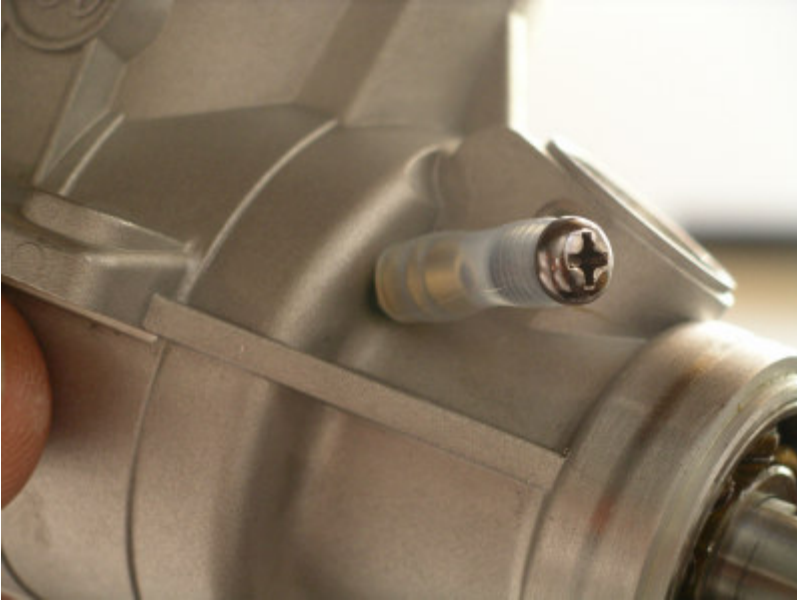
Capped grease fitting
